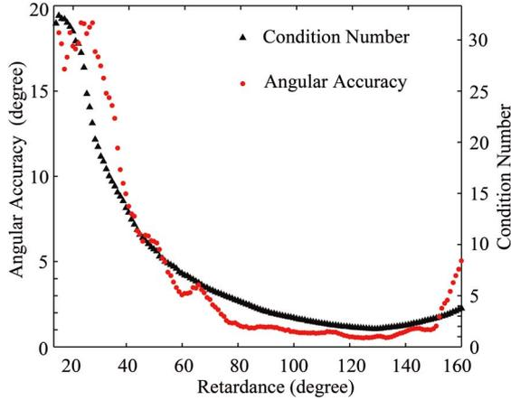
Fig. 4. CNs of the 146 annular subregions ranging from  $15^\circ$  to  $160^\circ$ , and the mean angular accuracies of the 60 measurements for the 146 annular subregions.
