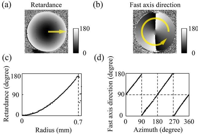
Fig. 2. Spatial distributions of linear retardance (a) and (c) and fast axis direction (b) and (d) of a GRIN lens 60 mm long, 1.4 mm in diameter, and 0.1 NA.
