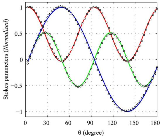
Fig. 5. Experimental (square marker,  $s_1$ ; circle marker,  $s_2$ ; triangle marker,  $s_3$ ) and calculated (red line,  $s_1$ ; green line,  $s_2$ ; blue line,  $s_3$ ) Stokes parameters corresponding to different incident SOPs, where in the PSG the polarizer is fixed and the wave plate is rotated  $180^\circ$  in 60 equal steps. The patterns on the CCD are recorded (see Media 1).
